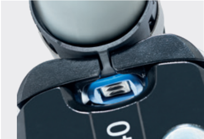
CLEAR TOOL GUIDE RIM The tool and pressing indicator fit together like a lock and key. This virtually eliminates the risk of a failed pressing sequence caused by incorrect positioning.
