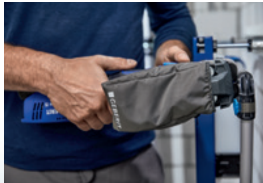
When pressing with the collection bag, the pressing indicators are collected directly and can be disposed of in bulk in the collection container.
